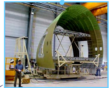
Sub-assembly of Section 11/12, Méaulte
